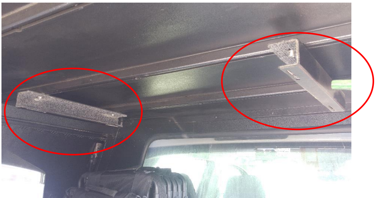
Figure 3: Table brackets installed
